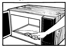
**1.** Empty the microwave oven and clean inside it with a soft, damp cloth. Check for damage such as misaligned door, damage around the door or dents inside the oven or on the exterior. If there is any damage, please do not operate the unit until it has been checked by an authorized Whirlpool<sup>54</sup> service technician and any repairs have been made.
