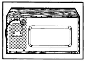
3. Do not block the vent or air intake openings on the rear of the oven. Blocking vent or air intake openings can cause damage to the oven and poor cooking results. Make sure the microwave oven legs are in place to ensure proper air flow.
