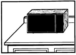
2. Put the oven on a cart, counter, table or shelf that is strong enough to hold the oven and the food and utensils you put in it. (The control side of the unit is the heavy side. Use care when handling.) The weight of the oven is approximately 35 lbs. (15.75 kg.).
