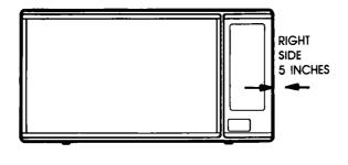
4. Do not install the microwave oven so that any part of it is flush with a wall, shelf or cabinet. Leave a total clearance of at least 5 in. (12.7 cm) around the oven for proper operation.
